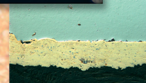
CC-12 mounted onto Olympus AX70 protective lacquer coating
