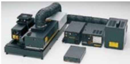
Laser combiner with Ar+HeNe (Red)+Kr laser systems
