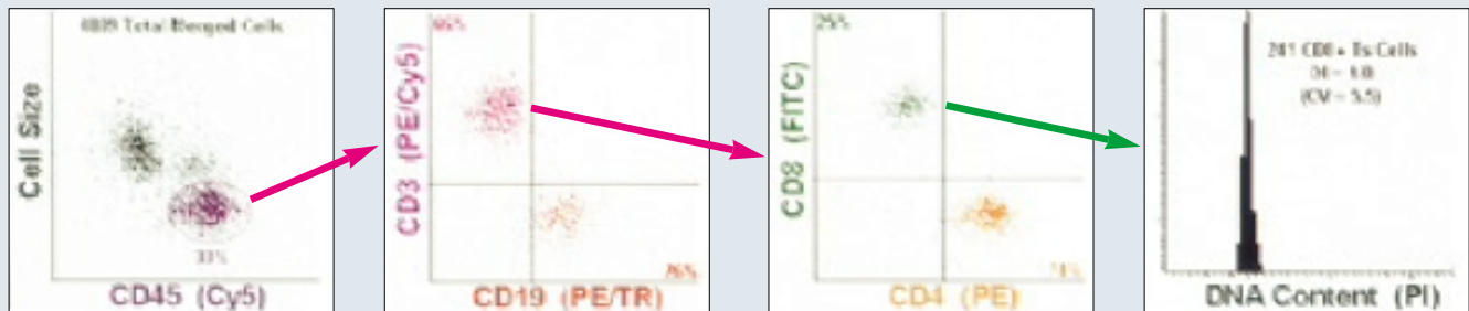
The above charts are 6-colour measurement examples, formed by merging 5-colour Immuno-fluorescence analysis data plus DNA-quantification using PI staining. Three different fluorochromes were applied to the same blood specimen in each scan pass, and data from each measurement were ultimately put together as a single data set for analysis.
